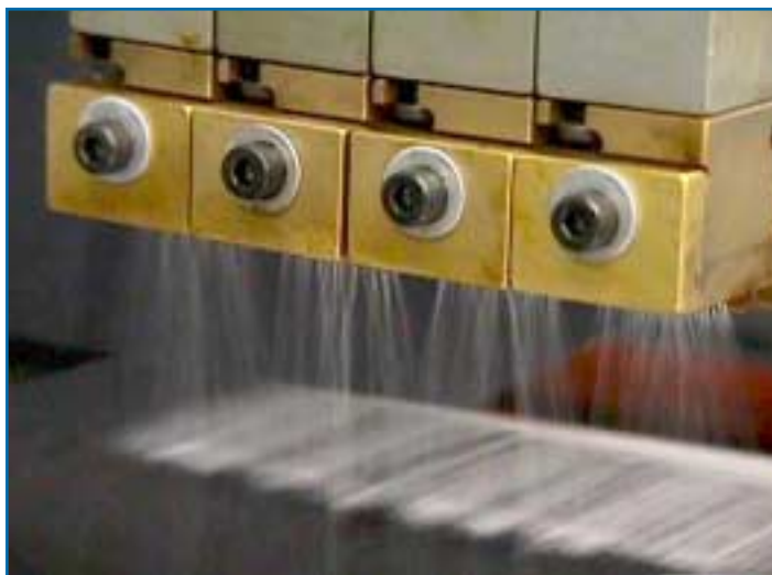
MB200 Applicator. The new Nordson MB200 sprays small-fiber hot-melt-adhesive patterns useful in a variety of diaper and sanitary-napkin applications.
