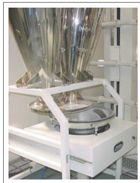
Fig. 2 Automatic Surge Hopper Lift Mechanism
