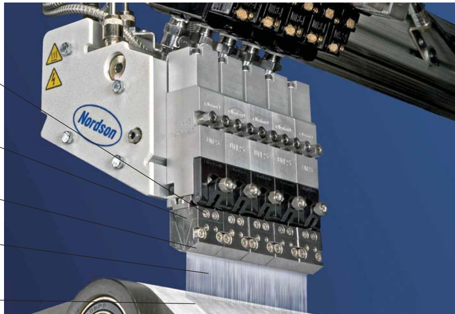
Universal applicator with UM25 modules and Control Coat nozzles
