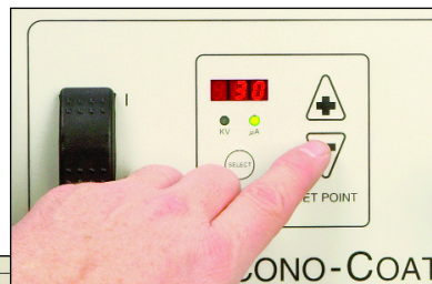
The Econo-Coat gun controller features easy selection/adjustment of kV and micro-amp setpoints.
