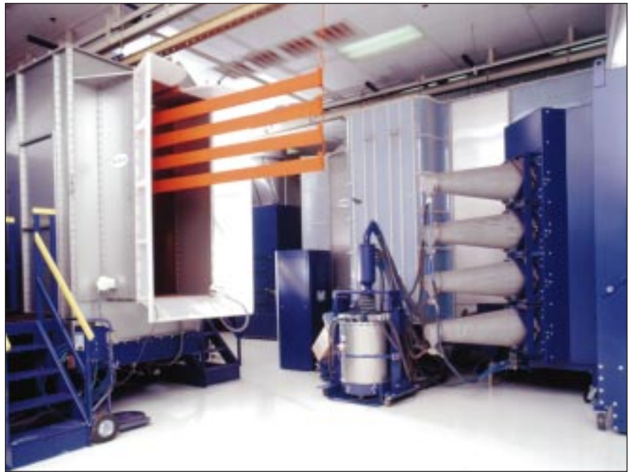
Powder Coating system with recovery system.
