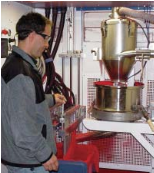
An employee observes the reclaim and feed systems. Both are designed to keep minimal powder in the booth at all times.
