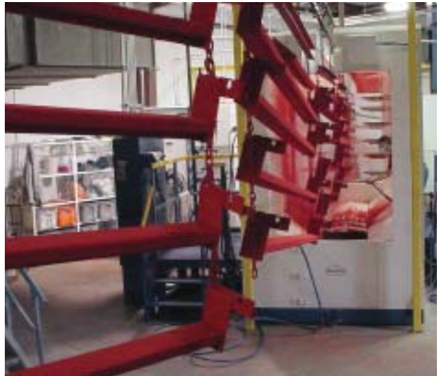
Parts are powder coated for Ridg-U-Rak, a North East, PA, pallet-rack manufacturer, at Cost Effective Coatings Inc., which also is in North East. (Photos courtesy of Nordson Corp.)
