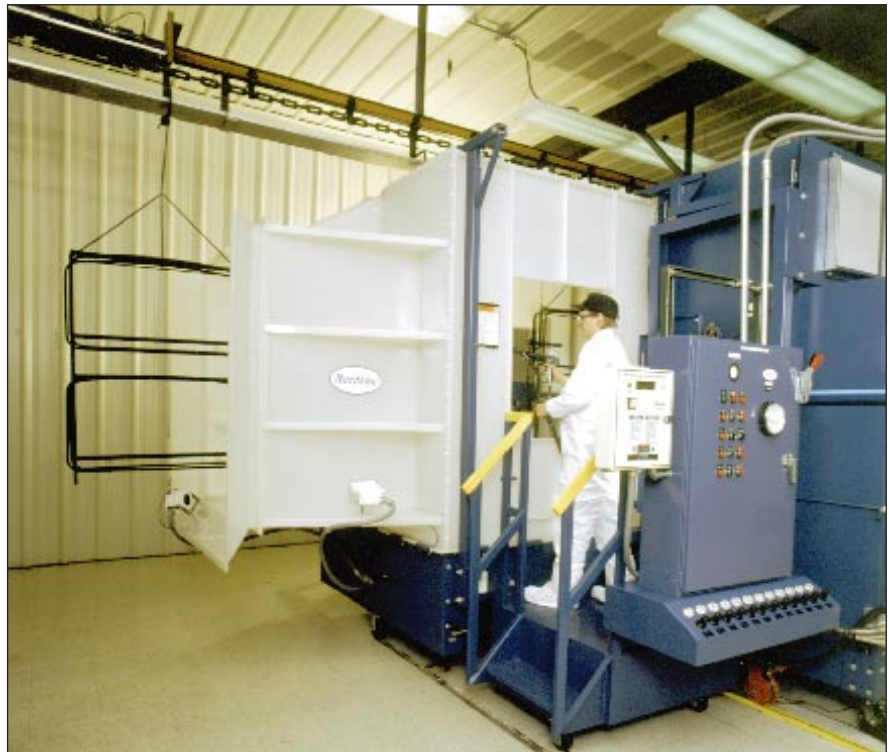
Before parts exit the booth, an operator uses manual touch-up guns for part recesses. (Photos courtesy of Nordson Corp.)
