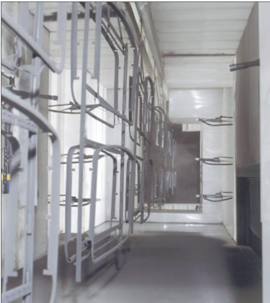
Automatic corona-charging guns apply powder coatings to parts. The system automatically recycles and reuses all powder that does not go onto the parts, boosting overall efficiency.
