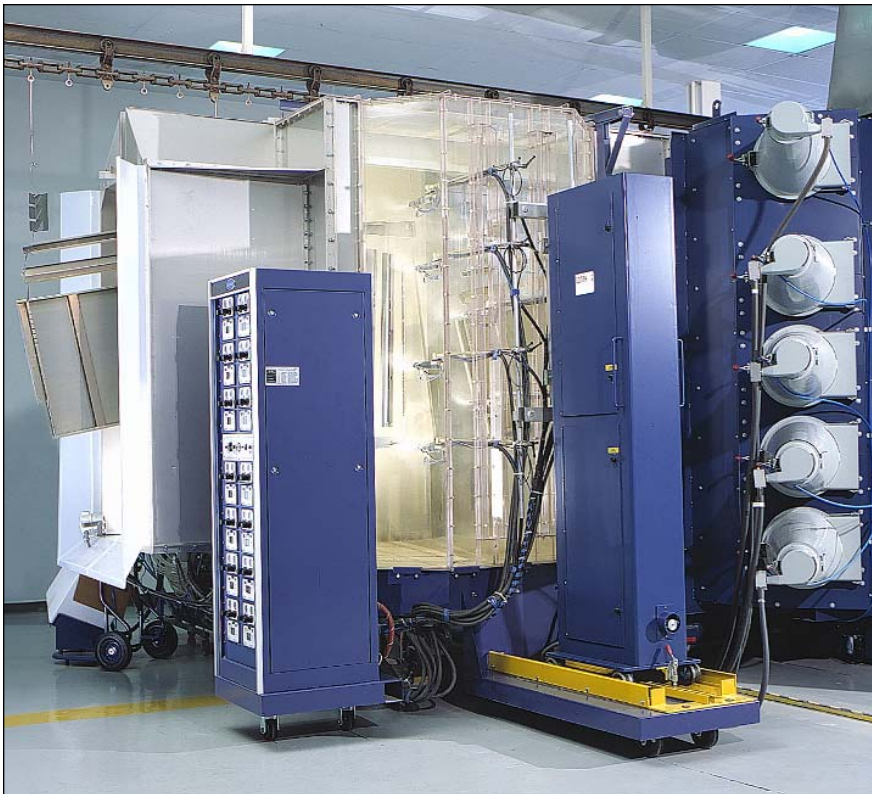
The roll-on, roll-off system enables Royston to change colors six or more times per day.
