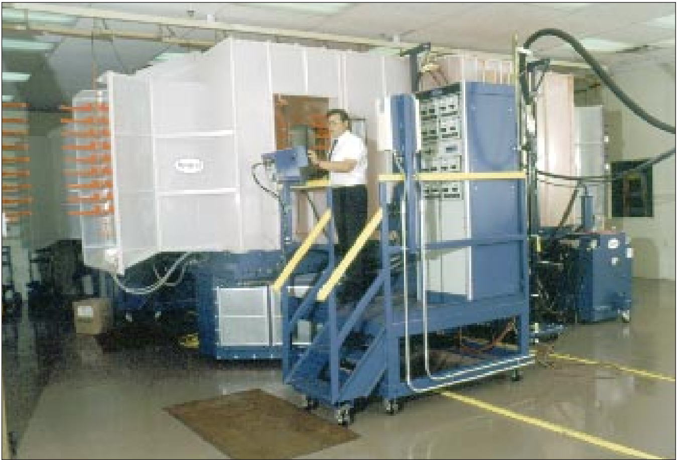
A temperature- and humidity-controlled room houses the automatic and manual powder booths, providing a clean working environment. (Photos courtesy of Nordson Corp.)
