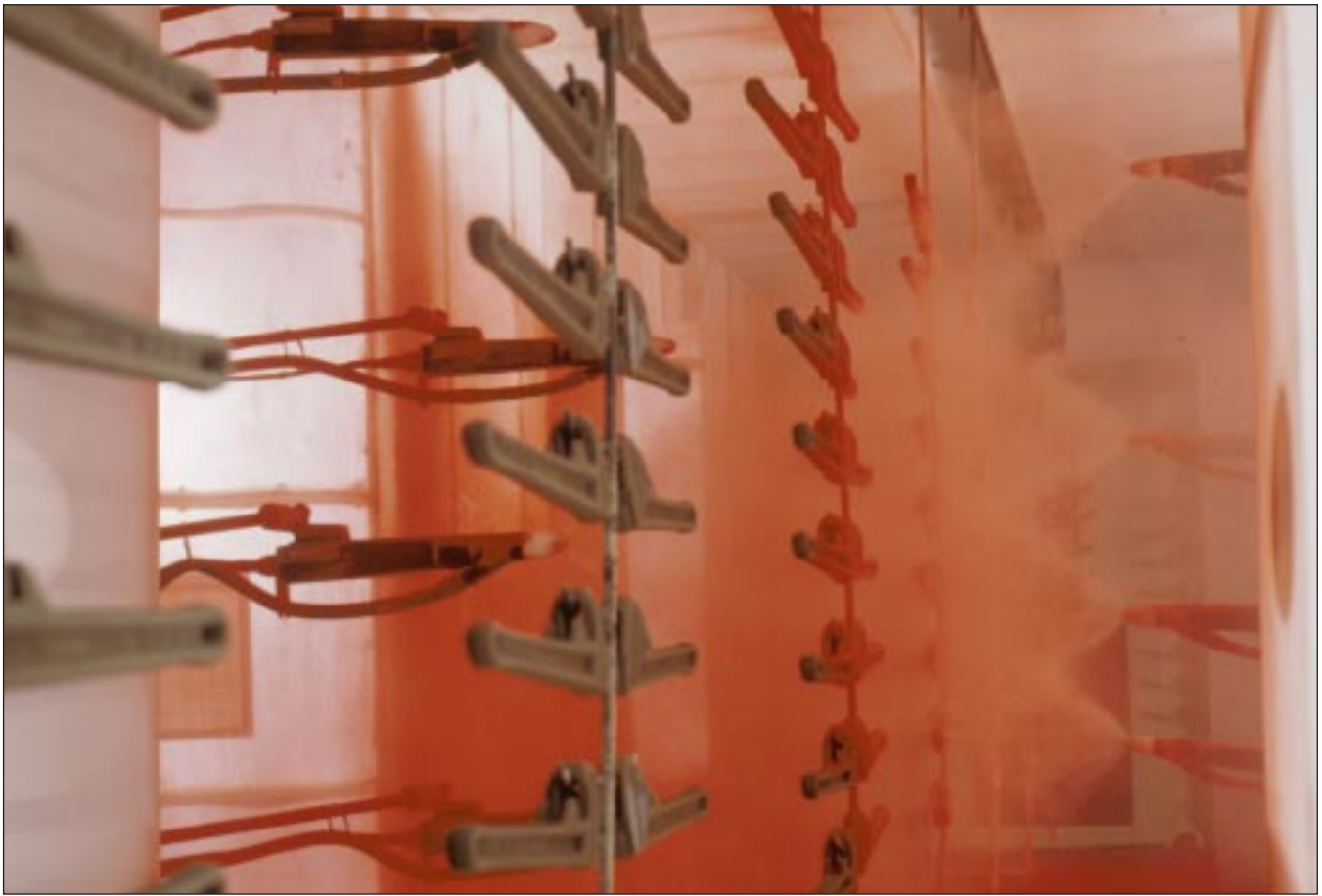
The Smart-Spray automated gun-triggering system uses multiple sensors at the entry of the booth to identify incoming parts on the rack and accommodate different part sizes. The increased efficiency of powder has eliminated 95% of all manual touch-up work required with liquid.
