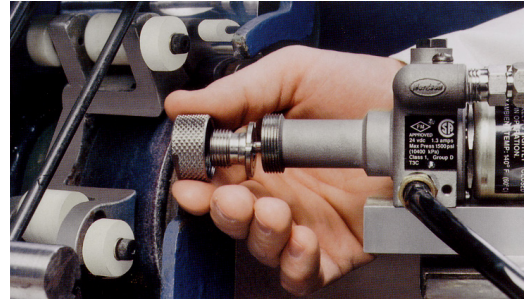
Module design facilitates easy on-line replacement of seat assembly in minutes.
